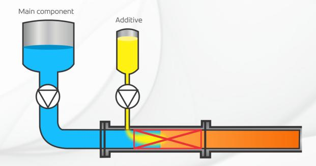
A static mixer is a precision engineered device for continuous mixing of fluids. They consist of an arrangement of mixing elements installed in a pipe or duct. They function without moving parts and are used to achieve specific dispersion and mixing in a continuous process. They are capable of mixing materials with equal or different viscosities and volume flow rates. The fluid flow is provided by pumping.
